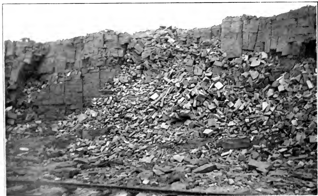
Ore Face, showing Characteristic Rhombohedral Cleavage, at Wabana Iron Mines.
